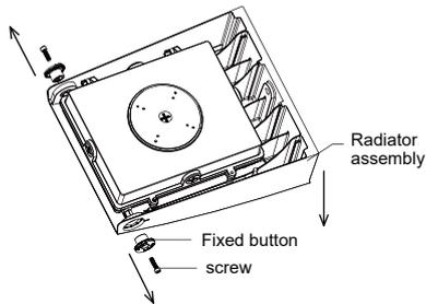
2. Use a screwdriver to remove the screw and remove the outer casing.
