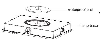
6. Put the input line and dimming line (if not, please ignore) from the embedded junction box through the lamp base and then screw the lamp base to the embedded junction box.
