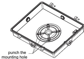
5. Tear off the adhesive paper of the waterproof pad and stick the waterproof pad to the lamp base.
