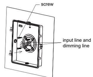
7. Install the upper half of the fixture on the lamp base, then use the threaded terminal to connect L/N/ ground wire, dim+/dim- (if not, please ignore) separately, and then plug the threaded terminals into the embedded junction box, adjust the switch to the required color temperature.
