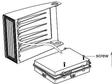
3. Unscrew the cover of the entry hole on the lamp base and remove the cover.
