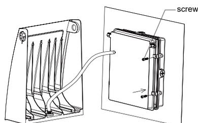
9. Install the heat sink assembly and tighten the screws and fixing knob with a screwdriver to complete the installation.
