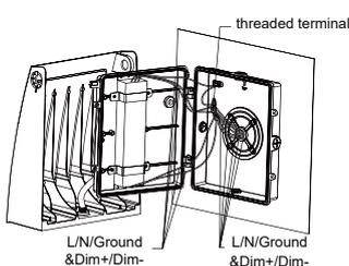
8. Screw the case with a screwdriver.
