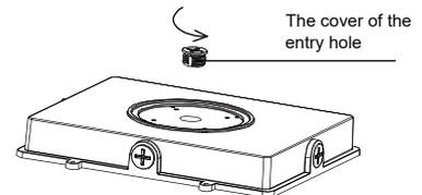
4. According to the embedded terminal box, punch the corresponding mounting hole on the light's mount.
